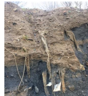
Picture 3. Sea eroding dredge spoil placed on shore as beneficial reuse. Courtown.
