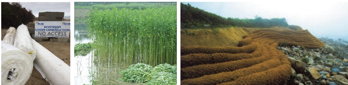
Figure 29. Coastal protection materials left to right: Plastic Geotextile underlay for rock armour and concrete blocks , : Jute plants, Coir logs used in coastal protection.
